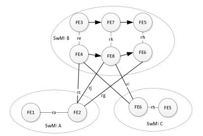
Figure 9: Functional model for ANF-ISIIC when the called user has migrated during the call to the forward switching SwMI
