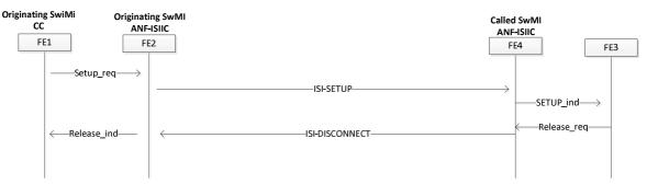
Figure 16: Information flow sequence - call rejected by the called SwMI
