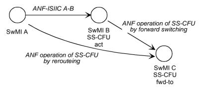
Figure A.1: Interaction with SS-CFU Forwarded-to user with home SwMI being SwMI B, having migrated
