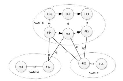
Figure 8: Functional model for ANF-ISIIC when the calling user has migrated during the call to the forward switching SwMI
