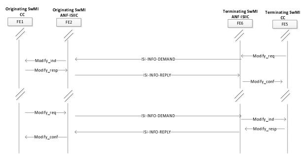
NOTE: The MODIFY request/indication information flow sends a request to modify the existing basic service into another one, and/or to change from duplex to half-duplex, or vice-versa, and/or to change the call duration.
