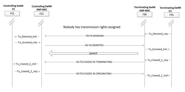
Figure 17: Information flow sequence - half-duplex operation
